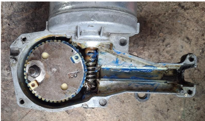
(3) Inside the wiper motor (drive pin relocated, note solder)
