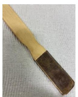
The **first stage** involved the clean-up of the rusted areas with the use of a thin piece of wood (something akin to a 30cm ruler) to which I super-glued a strip of Norton P240-J emery paper; special in that it had a cotton material (not paper) backing, that when torn, would tear straight. However, it did take a while to do this work, as it does need to be done carefully, in order to prevent unnecessary scratching of the good chrome areas.
