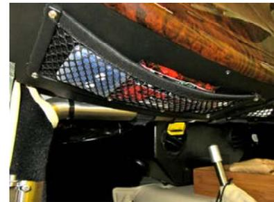
steering wheel but... it was in the way of the passenger's knees anyway! You will also note a wooden box I found at a local homewares store (this one is bamboo) that fit very nicely on the top of the transmission. I used a couple of rubber blind nut fasteners to attach it to the unused “radio” plate in the heater box. You can see where the second Hobie panel is located in this photo as well. Amanda uses the one under the glove box, I use the one on top of the transmission tunnel.
