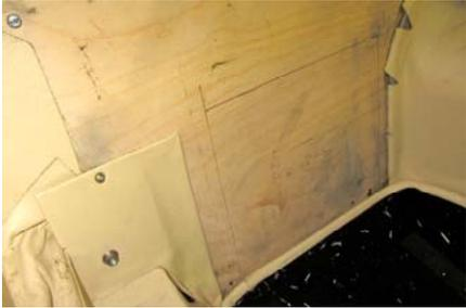
convenient to duplicate this option but what was of interest was access through the vertical panel. As I already had a shallow lockable "box" that could be used (red top is visible in the photos) I mocked up a larger cardboard template using the "red" lockable box as the access port. Once happy with the fit I translated the cardboard box into a steel structure (mild 1mm steel sheet from an old dishwasher), cut
