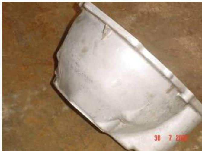
Bellhousings: The alloy bellhousing. Also suitable for a 5-speed conversion and much lighter than the cast unit.
