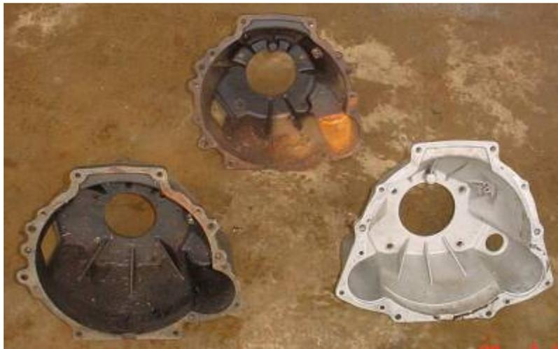
Comparison of bellhousings: Capri (left); cast bellhousing (centre); alloy bellhousing (right). Notice the cutout for the fork is much lower in the later types. Some modification of the clutch linkage is necessary to accommodate this change if you are changing from a Capri setup.
