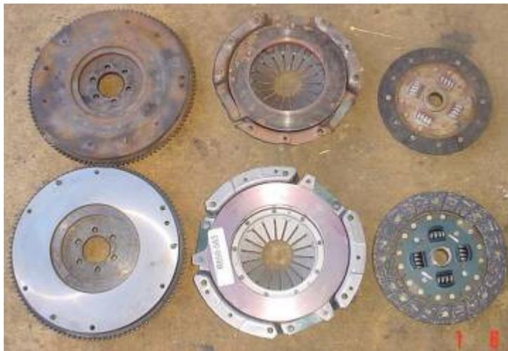
Flywheel options: A complete 195mm setup (top) and 215mm setup (bottom). Both will connect a 1600 to a Sierra 5-speed. Note the different location of the dowels and holes on the flywheels.
