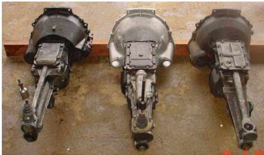
Some gearbox options: Single rail and Capri bellhousing (left); 5-speed with alloy bellhousing (centre); 4-speed "type B" with cast bellhousing (right). Note that all are the same overall length and have the gearlever in the same position.
