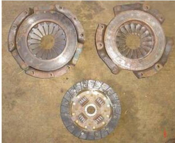
195mm pressure plates: 6 bolt (left) and 3 bolt (right). The driven plate (bottom) will suit either type.
