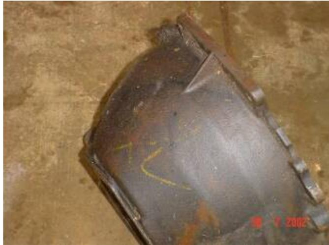
Bellhousings: The cast bellhousing. This is suitable for the 5-speed and freely available.
