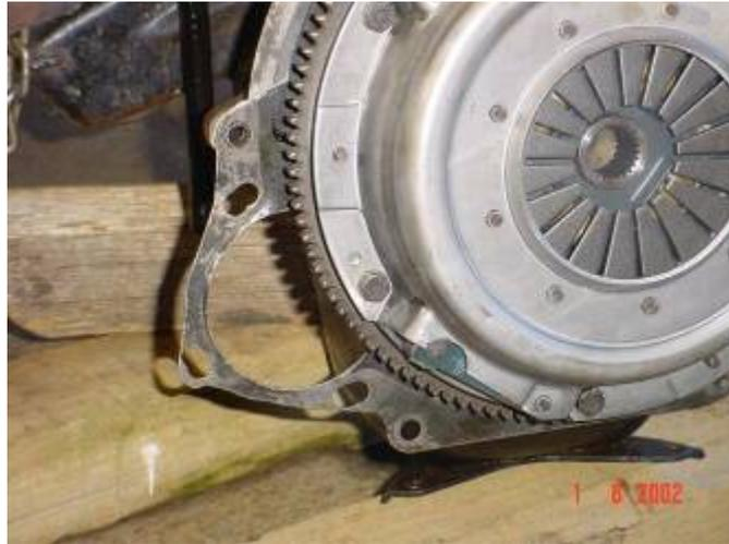
Fitting the starter motor: Modifications to the plate between the engine and the bellhousing to accommodate the slight change in starter location.
