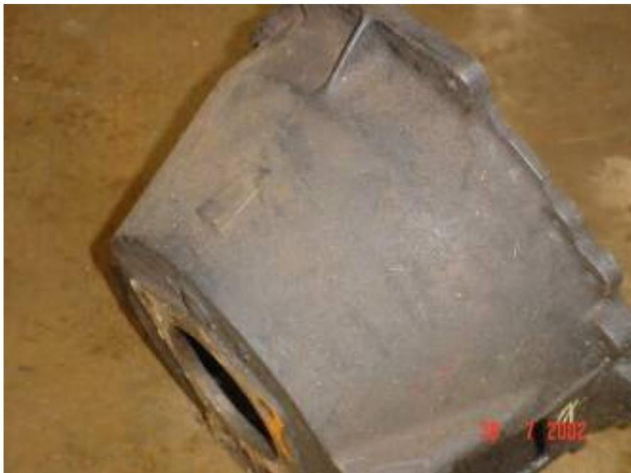
Bellhousings: The Capri bellhousing. Note the rectangular protrusion on top of the bellhousing for identification. This bellhousing will not attach to the 5-speed gearbox.
